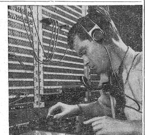
1. Here's the "ear"-an electronic ear called a low insulation alarm. It listens for underwater cables to signal they're in trouble. Right now the meter shows something's happened . . . perhaps a sharp submerged rock has cut a cable . . . and vigilant telephone men using another testing device locate the break that may be miles away.
