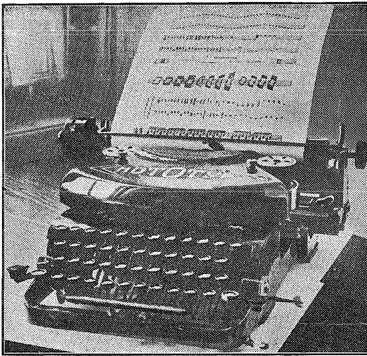
SAY IT IN MUSIC! The first practical typewriter designed to write musical compositions. It was perfected by Gustav Rundstaddler, has 44 keys, and by delicate spacing controls, a musician can write a musical score as easily as a letter.
