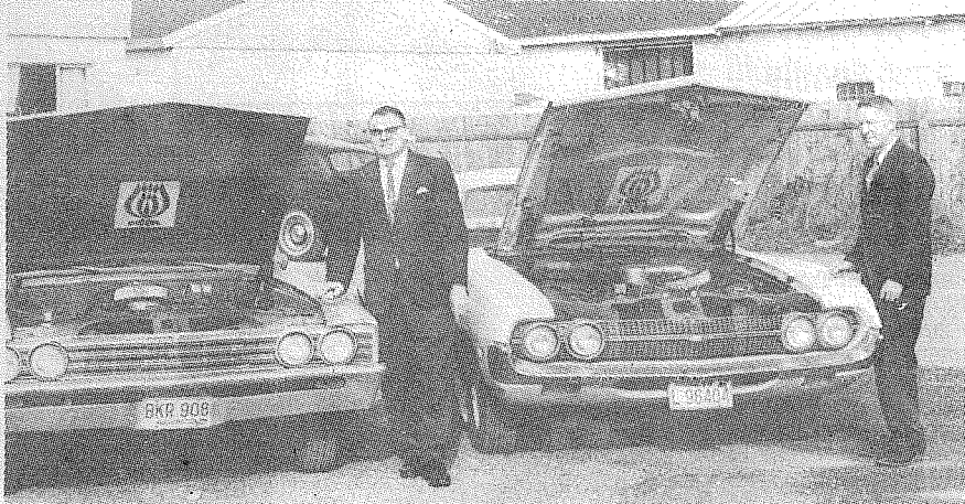
PROPANE POWERED. Doxel Redi-Gas employees early this week displayed two vehicles that have recently been converted to propane carburation. The Parkland firm at 14012 Pacific Avenue says the propane units help cut air pollution in addition to reduce engine operating and maintenance costs.
