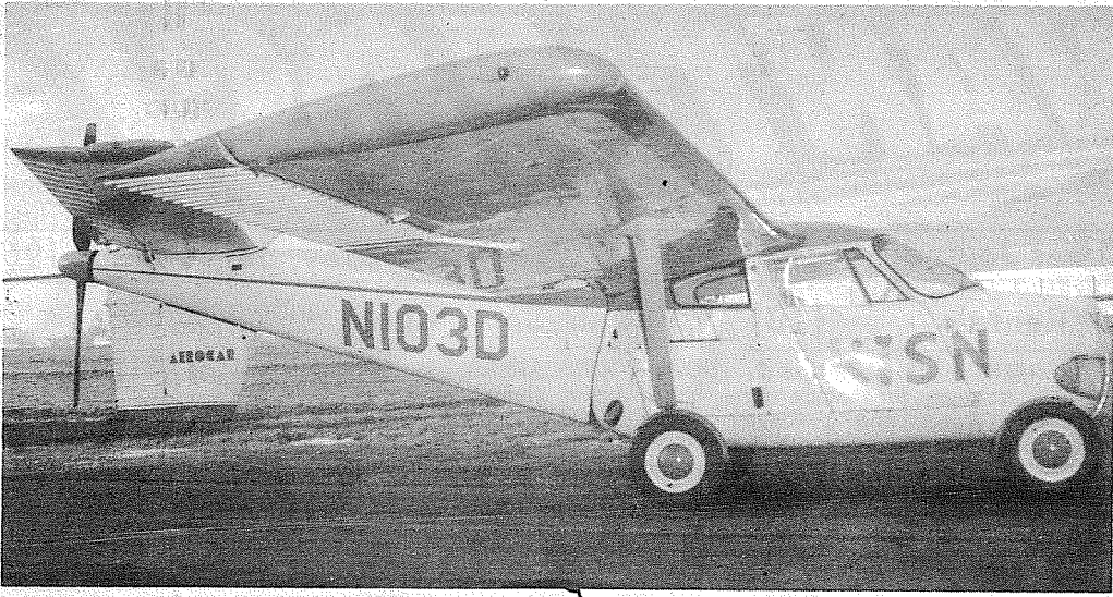
IT'S A CAR — IT'S A PLANE — it's a revolutionary concept in traveling made practical in the Aerocar shown above. When the traffic congestion gets this driver's goat he just gives it the old air! This is the vehicle that can be a complete FAA approved light plane - a combination plane and car, or, wings removed, a complete little coupe for around town travel. —Times Journal Photo
