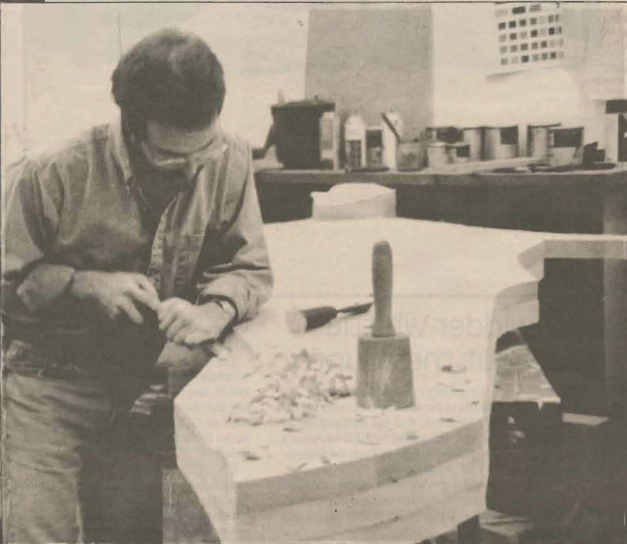
Tim Bergren gouges the initial strokes into the current commission. The carving process can take anywhere from two weeks, to several months to complete.
