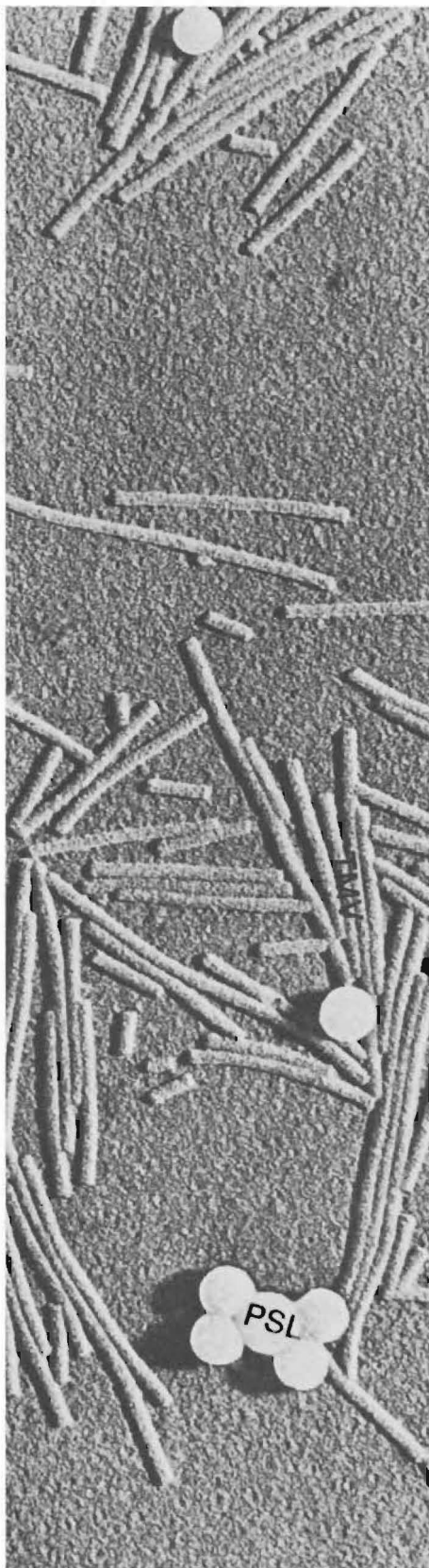
Chromium shadowed tobacco mosaic virus (TMV) in the presence of 880A Polystyrene (PSL) calibration spheres (X52,000).
